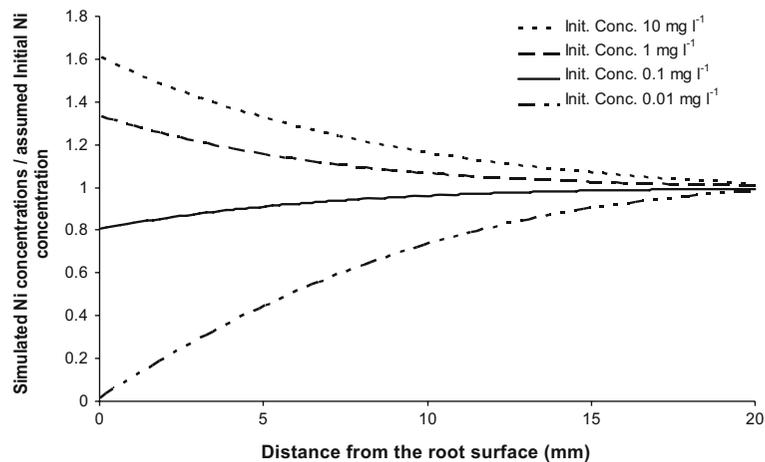
**Fig. 9** Simulated  $\text{Ni}^{2+}$  concentration profile as a function of distance from root surface assuming various initial concentrations.  $\text{Ni}^{2+}$  concentration profiles were normalized by dividing by the corresponding initial concentration. All other parameters were kept constant
