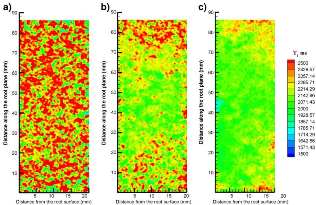
**Fig. 5**  $T_1$  maps at horizontal cross-sections of the rhizobox at  $t=11$  h when the water level dropped in the rhizobox: **a)** 1st slice from top where it was unsaturated, **b)** 2nd slice partly saturated, and **c)** 4th slice completely saturated
