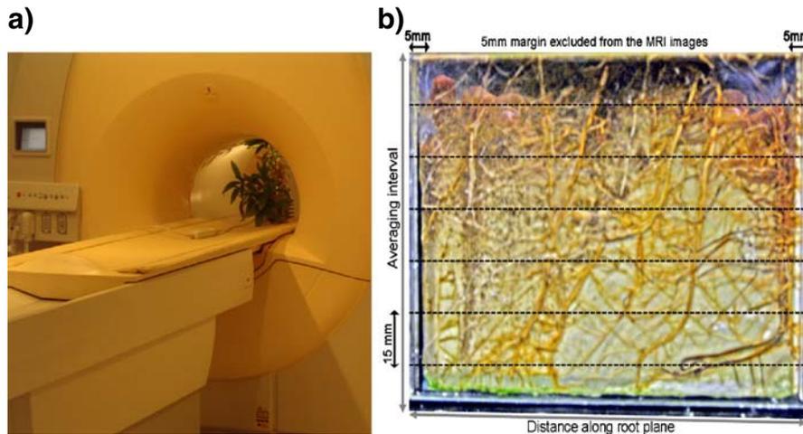
**Fig. 3** A view of the rhizobox placed inside the MRI machine (a) and the root distribution pattern before the Ni<sup>2+</sup> uptake experiment (b). The broken lines indicate the 15 mm thick slices into which MRI signal was recorded
