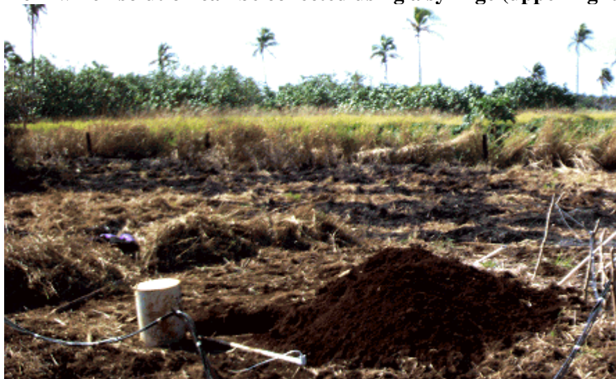
Figure 3. The flux meter about to be buried in a pit where it can record drainage and allow sampling of the leachate.
