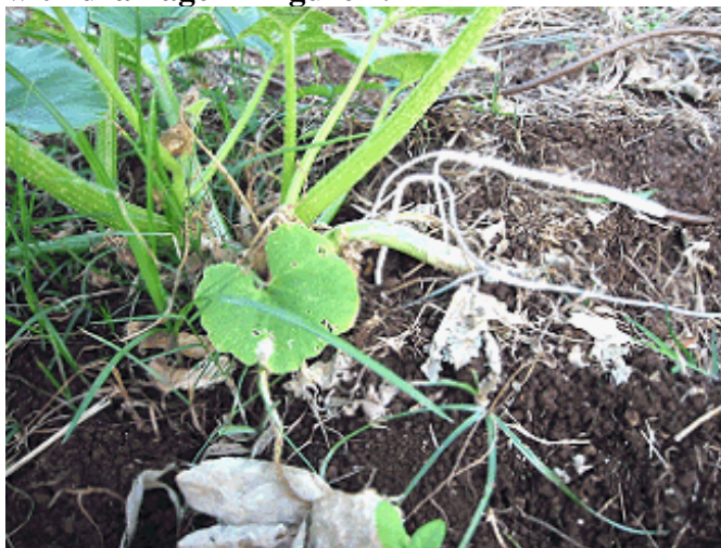
Figure 6. The water-use of the squash pumpkin was measured using heat-pulse monitoring of the sap flow in the stems of the plant. The white wires in the stem on the right of the photo are connected to a heater needle (centre), and two temperature sensors either side.
