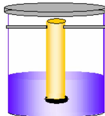
Figure 1. The experimental set-up of the CCA leaching study on H4-treated timber posts with sealing of the bottom.
